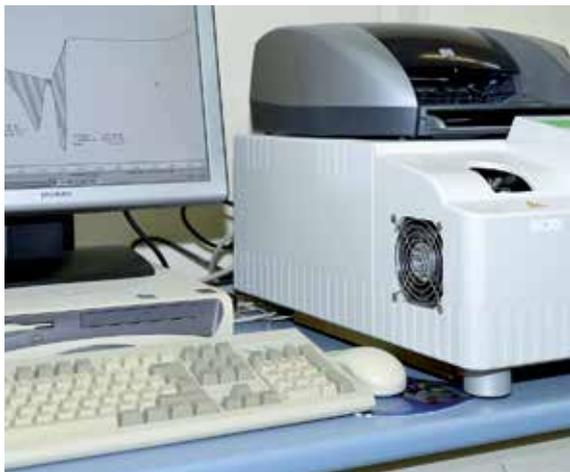
The Differential Scanning Calorimeter (DSC) analyses the thermal behaviour of a material over its total mass, i.e. the total thickness. It cannot provide any information about the surface of a material, but it determines the percentages in its composition very accurately.
