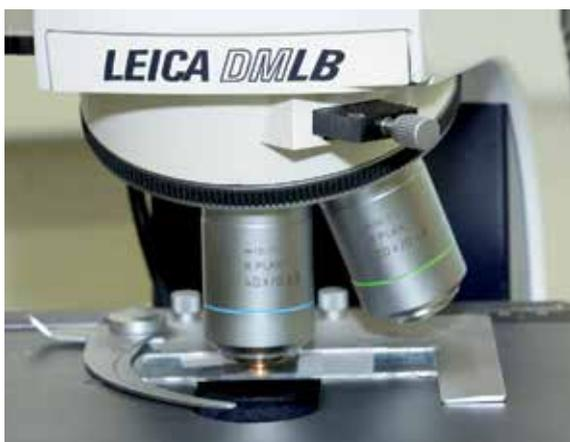
Our Microtome cuts wafer-thin samples out of a compound which then can be analysed under a special microscope with regards to their composition. The resolution of this high-performance instrument allows for the recognition of the finest layers of ink and glue.
